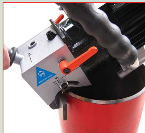
Ideal for beveling pipe 6 1/4" OD and larger.
